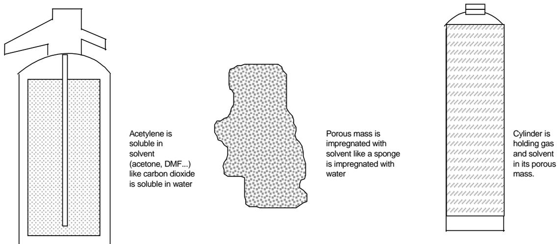
The cylinder shell itself is made of steel and is either of extruded or welded construction. All cylinders are fitted with valve outlets and have a left hand thread (because acetylene is a flammable gas) or a special connection.
