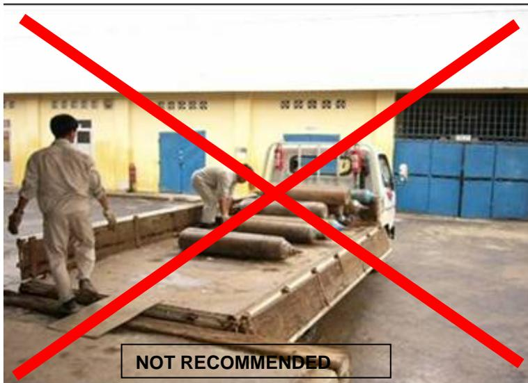
Figure 3 - Personnel handling horizontally loaded cylinders
