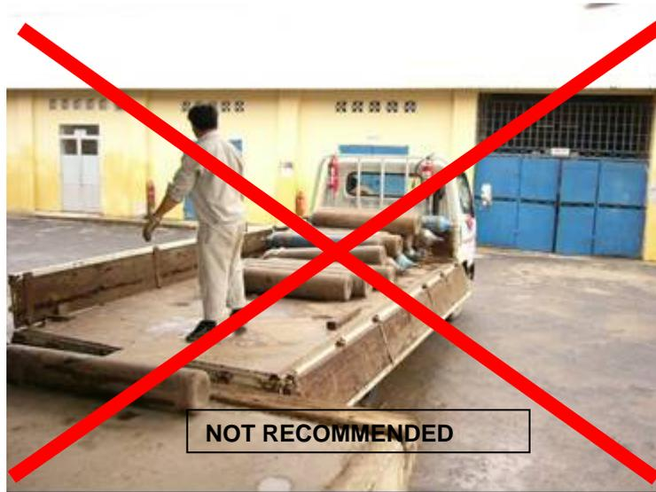
Figure 4 - Cylinders rolling during unloading
