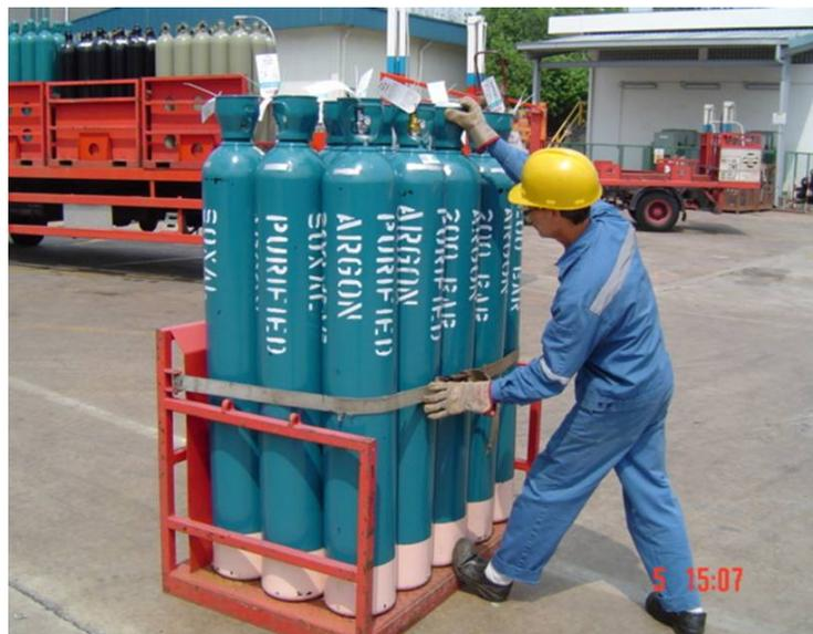
Figure 12 - Cylinders secured with a strap inside a pallet
