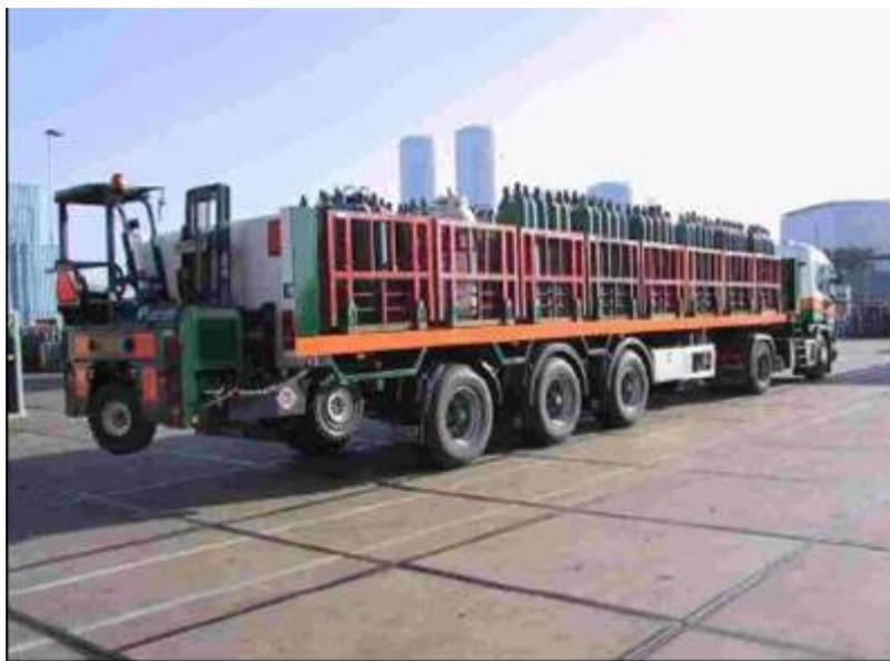
Figure 13 - Cylinder truck with forklift
