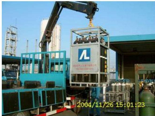
Figure 11 - Cylinder truck with crane
