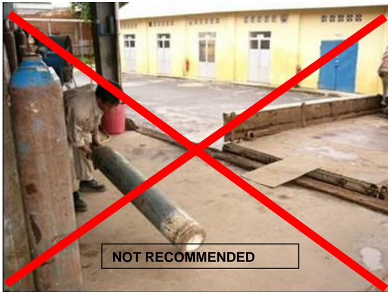
Figure 2 - Bringing a cylinder to vertical position
