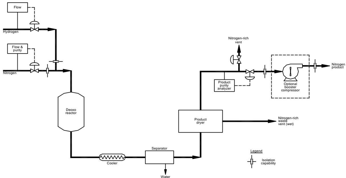
**Figure 12—Deoxo flow diagram**
