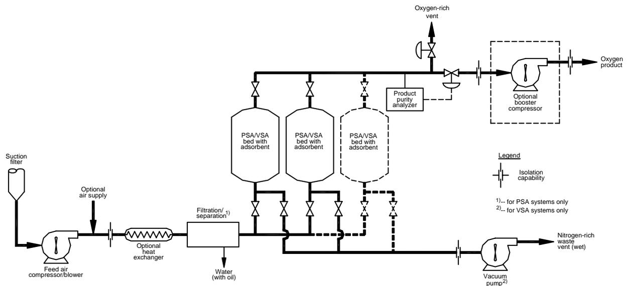
NOTE—The number of vessels can vary from one to four or more. The dotted vessel shown in Figure 1 is meant to indicate this variation in the number of vessels.
