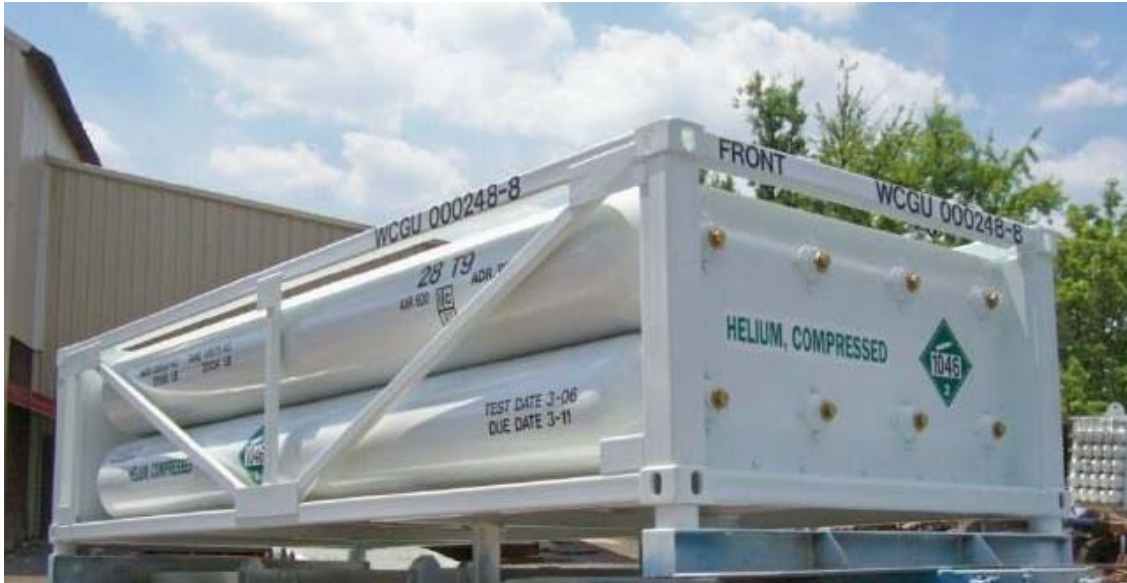
Figure C-5—Multiple element gas container (MEGC) (20 ft for compressed and liquefied compressed gas)
