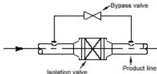
**Figure 3 Example for a bypass system**
