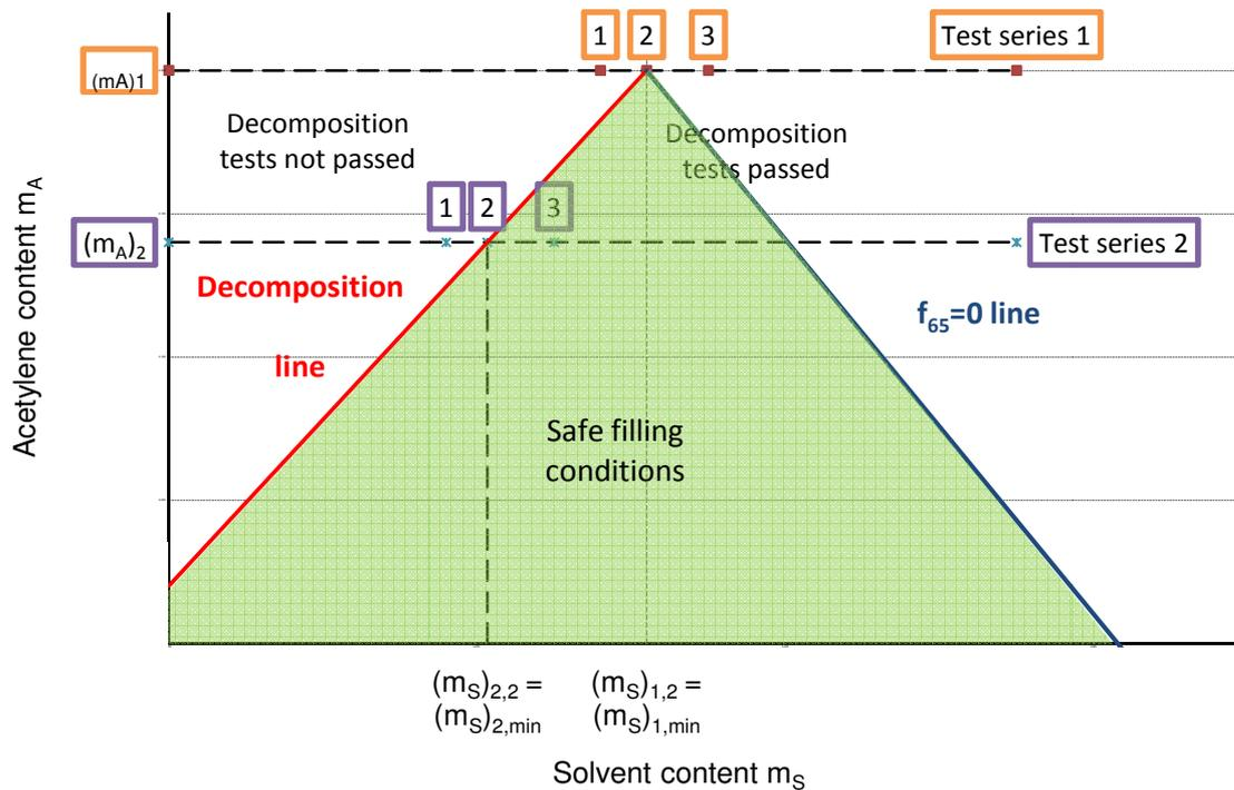
Figure 2: Determination of the safe filling conditions
