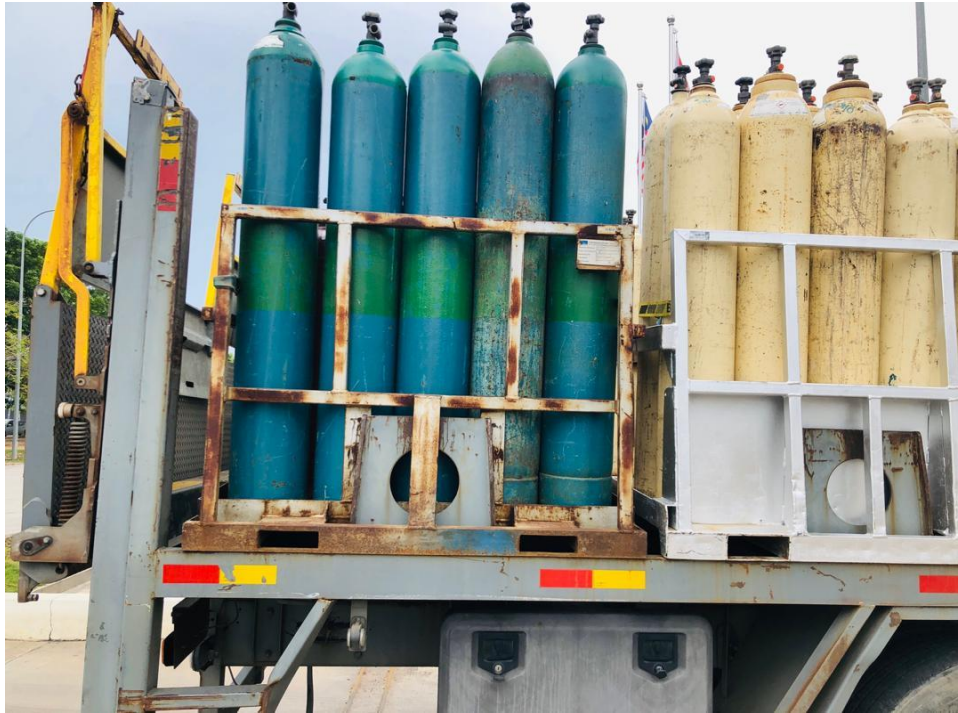
Figure 6 - Vehicle with cylinder pens and load secured by straps
