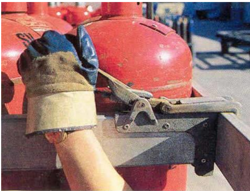
Figure 7 - Transverse slats with rapid clamping device
