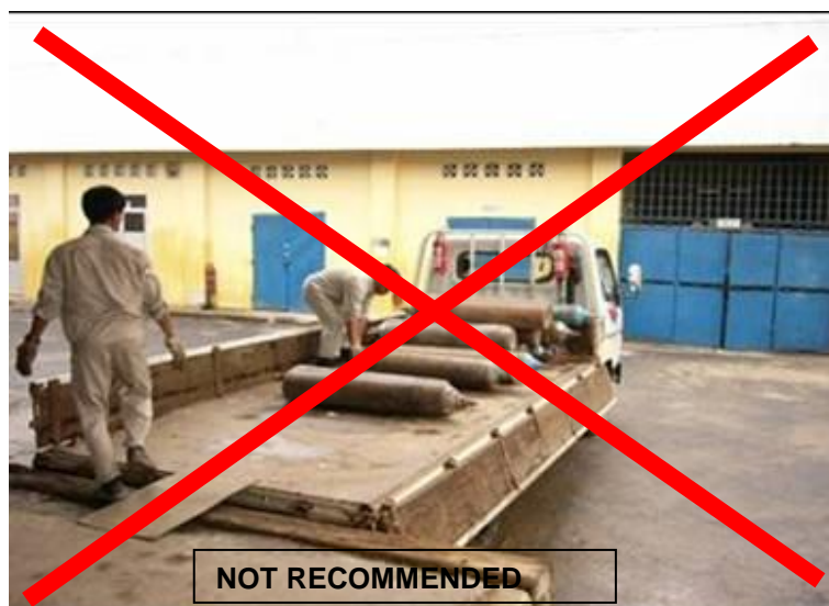
Figure 3 - Personnel handling horizontally loaded cylinders
