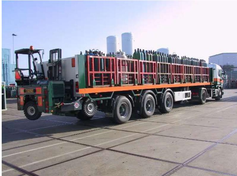
Figure 13 - Cylinder truck with forklift
