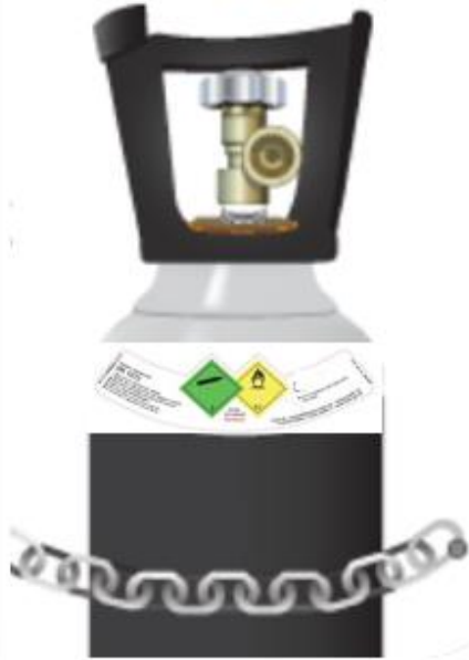
Cylinder Properly Secured
