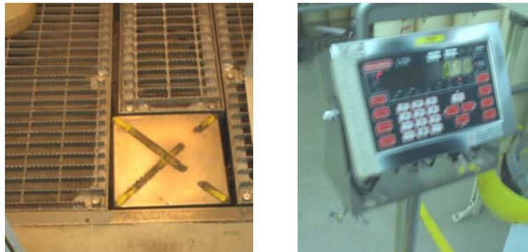
Figure 9 - Weigh scale platform and indicator
