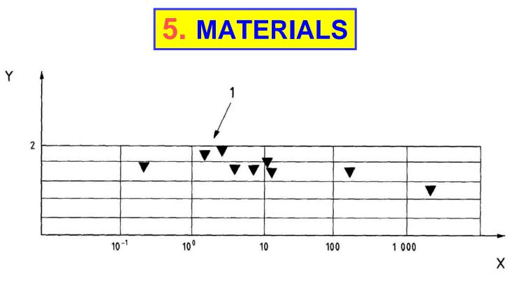
X. Pressure rise rate (bar/min) Y. P<sub>r'He</sub> / P<sub>r'H2</sub>
