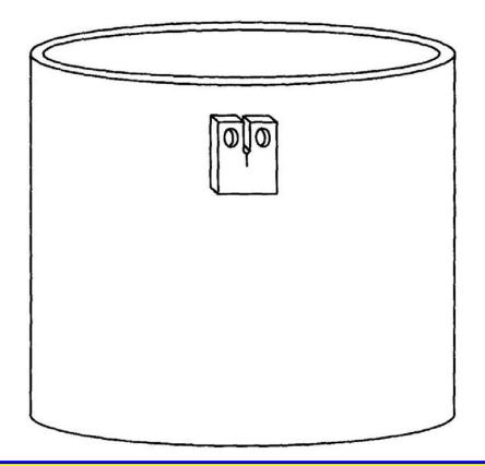
**Compact tension test piece : type and orientation**
