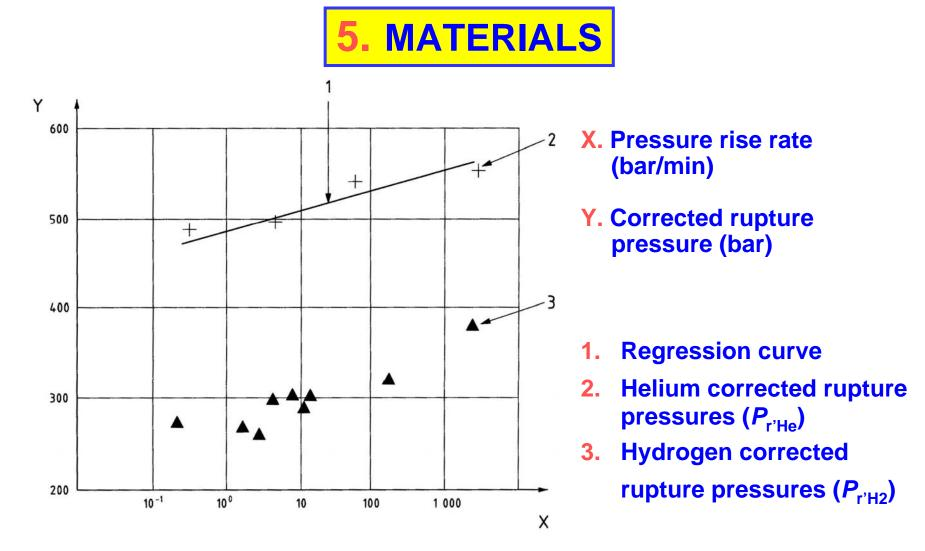
Examples of hydrogen and helium corrected rupture pressure as a function of the pressure rise rate
