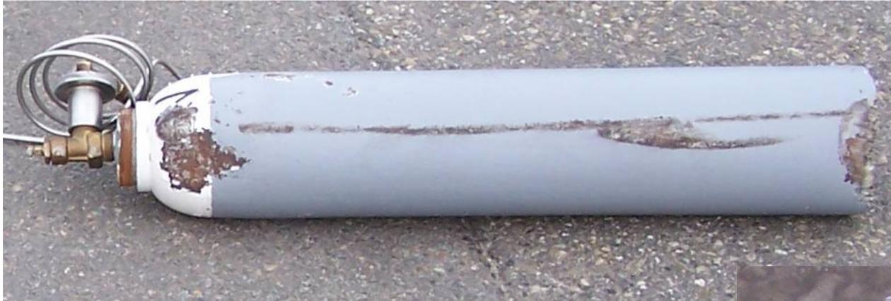
**Originally 13.4 litre CO2 cylinder, base cut, barrel shortened and base welded to barrel to look like a 10 litre cylinder**
