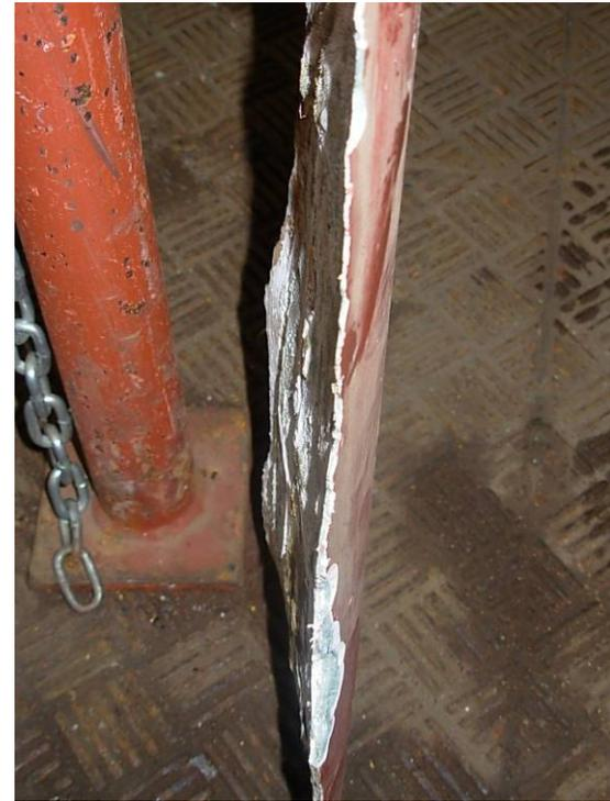
**Damaged acetylene cylinder “repaired” with plaster**
