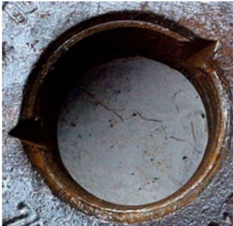
a) Hairline crack without visible sidewalls
