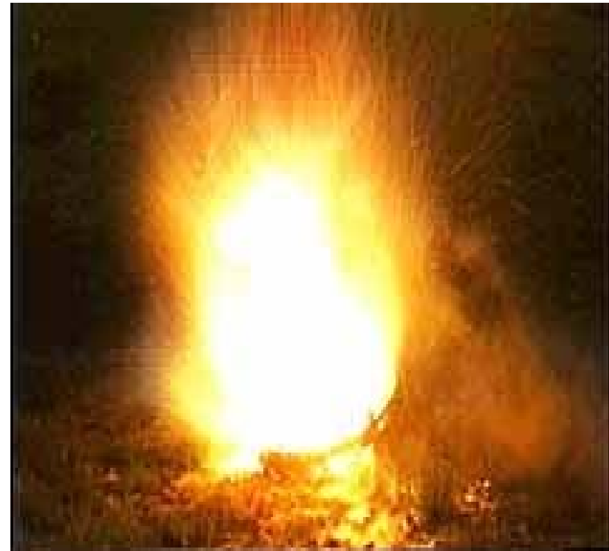
Effect of adding LOX to a charcoal fire
