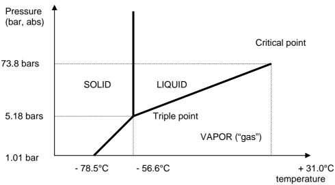
Diagram 1: section of CO2 pressure-temperature diagram
