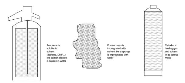
The cylinder shell itself is made of steel and is either of extruded or welded construction. All cylinders are fitted with valve outlets and have a left hand thread (because acetylene is a flammable gas) or a special connection.
