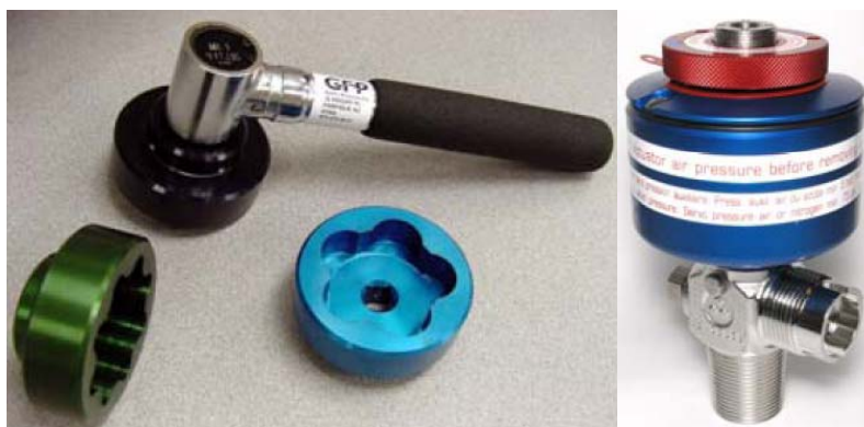
Figure 5.3.1 A typical handwheel torque wrench and an air actuated valve with a DISS outlet
