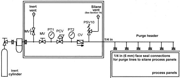
NOTE—The purge gas panel is allowed to be connected to one or more process gas panels with the purge header. Figure 9 has been provided to illustrate the concepts described in the text of the standard. The figure is schematic in nature. It is neither to be interpreted as a design document nor is it intended to restrict alternate designs. For instrument nomenclature, see Figure 1.
