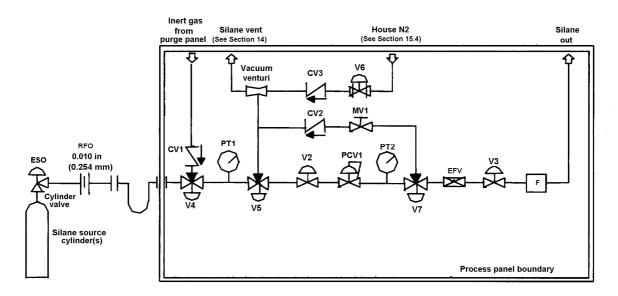
NOTE—The ESO valve is allowed to be located on the cylinder or on the pigtail close coupled to the cylinder. Figure 5 has been provided to illustrate the concepts described in the text of the standard. The figure is schematic in nature. It is neither to be interpreted as a design document nor is it intended to restrict alternate designs. For instrument nomenclature, see Figure 1.
