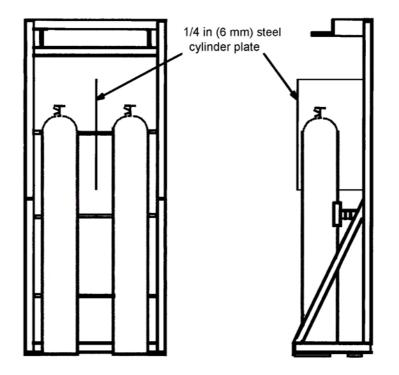
NOTE—The plate is designed to prevent flame impingement from the valve source to the adjacent cylinder. The plate shall be extended below the centerline of the valve a minimum of 18 in (460 mm). Figure 2 has been provided to illustrate the concepts described in the text of the standard. The figure is schematic in nature. It is neither to be interpreted as a design document nor is it intended to restrict alternate designs.
