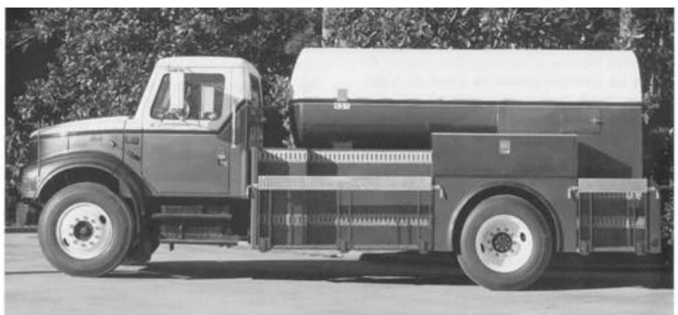
Figure 9—Liquid carbon dioxide cargo tank (straight truck)
