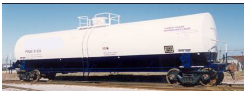
Figure 7—Liquid carbon dioxide tank car
