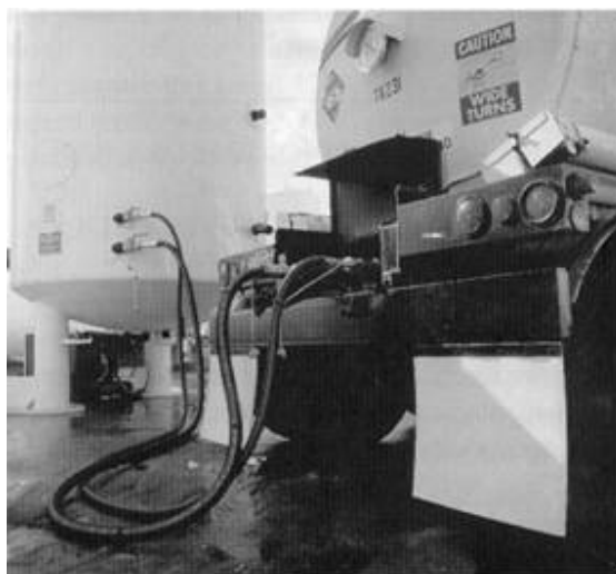
Figure 14—Bulk liquid transfer hose
