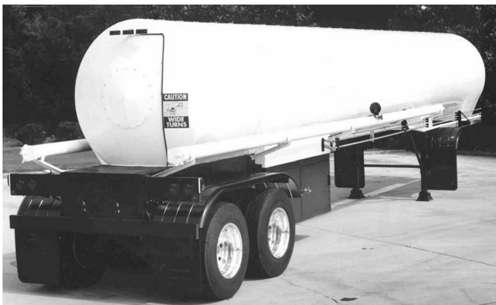
Figure 8—Liquid carbon dioxide cargo tank
