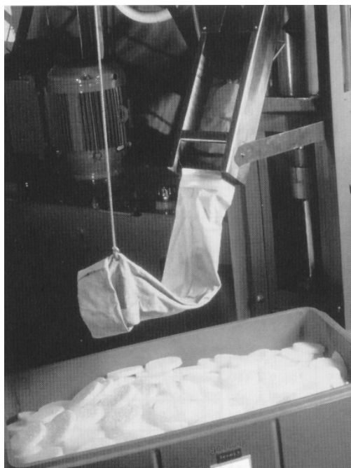
Figure 3—Production of dry ice disks for airline food module refrigeration
