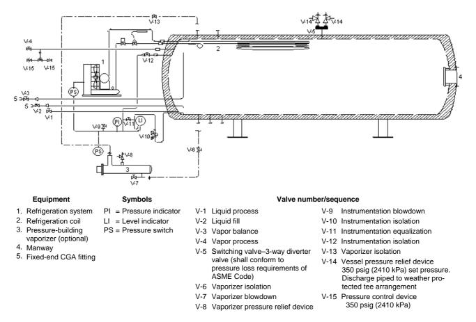
Figure 12—Typical piping schematic for carbon dioxide storage system
