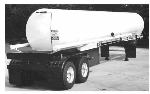
Figure 8—Liquid carbon dioxide cargo tank
