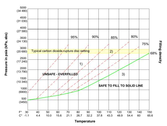
NOTE—This chart is based upon a cylinder filled to its correct maximum liquid carbon dioxide capacity of 68% of the total volume (water weight capacity). An overfilled cylinder obviously experiences enormous internal pressures from expansion of the liquid carbon dioxide as it warms to higher temperatures after filling.
