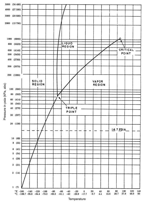
Figure 1—Carbon dioxide phase diagram
