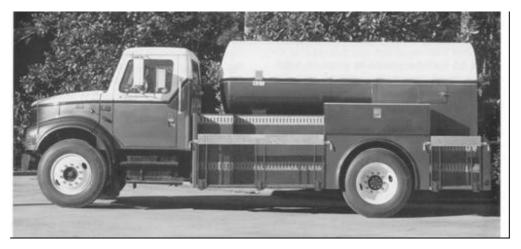
Figure 9—Liquid carbon dioxide cargo tank (straight truck)
