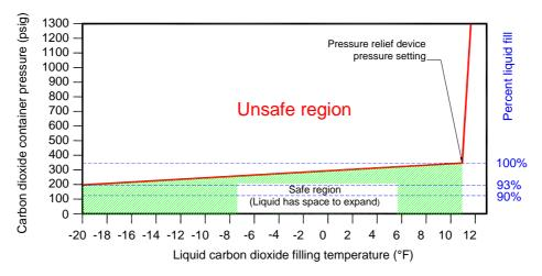
Figure 4—Safe filling volumes for 350 psig carbon dioxide containers
