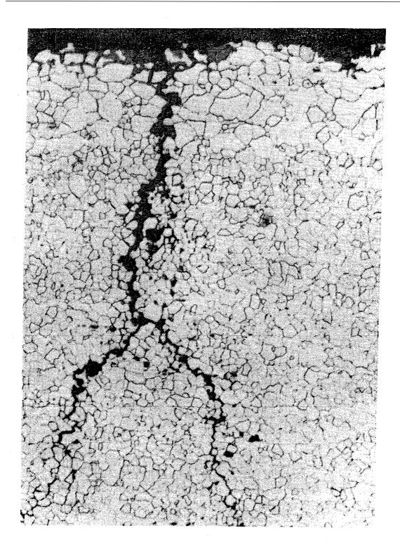
Figure 1 - Stress Corrosion Cracking of a brass valve
