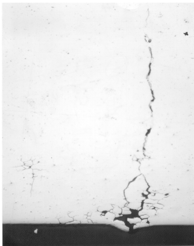
Figure 1 – HW Cylinders (AA 6061) Fatigue crack initiated from a corrosion pit. Magnification X 125
