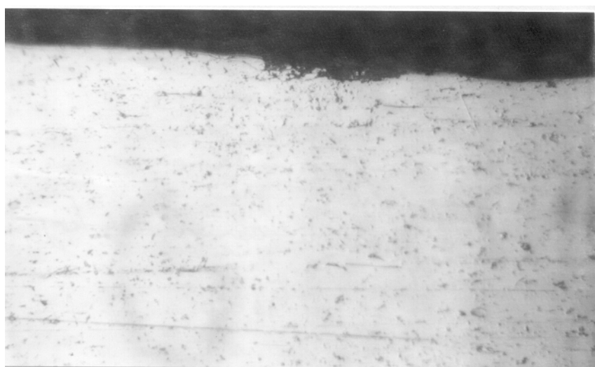
Figure 2 - AA 7060 Cylinder Metallographic examination according to the intercrystalline test as per EN 1975. Magnification X 300
