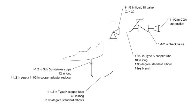
Figure B-2—Sample calculation 1—fill line sketch
