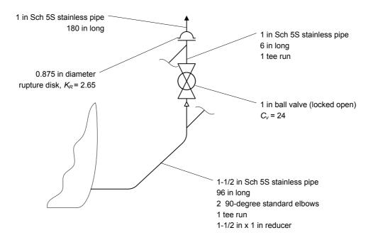
Figure C-1—Sample calculation 2—relief line sketch
