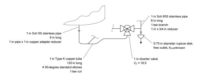
Figure B-1—Sample calculation 1—relief line sketch
