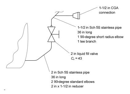
Figure C-2—Sample calculation 2—fill line sketch
