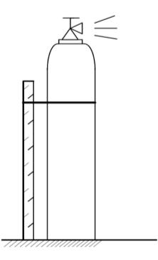
4A.2 Description of method: Gas is discharged directly from the container valve to the atmosphere.
