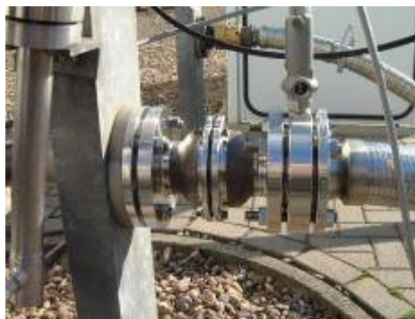
Figure 1 Typical breakaway coupling for liquid filling
