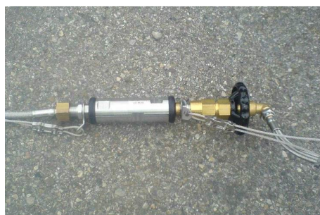
Figure 2 Typical breakaway coupling for gaseous filling
