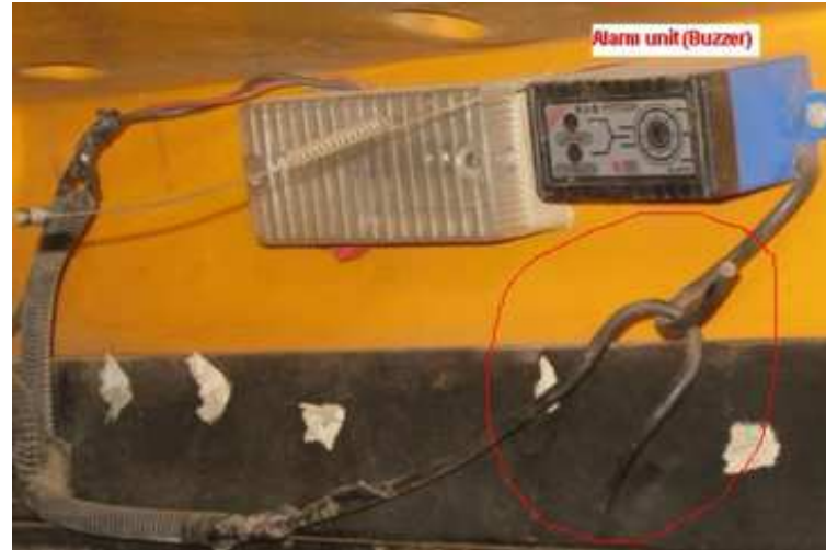
Electrical wire to the alarm was cut
