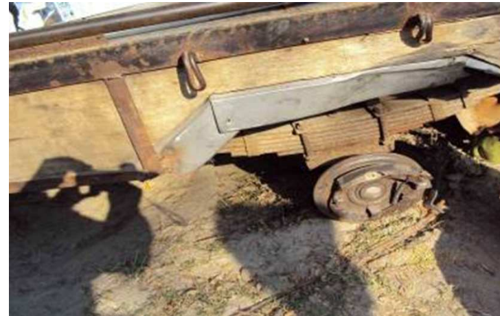
Third party three-wheel vehicle with broken rear axle
