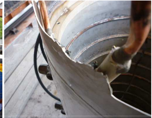
Ruptured buffer vessel viewed from different angles, pictures 1 - 4
