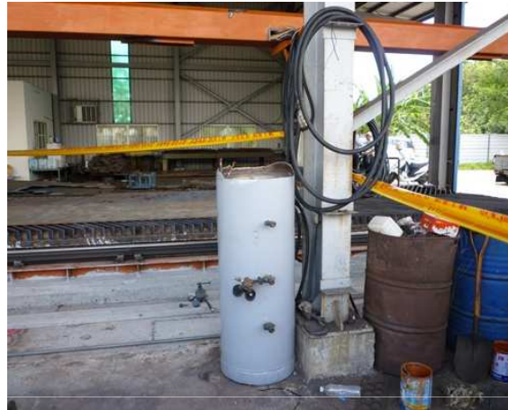
Ruptured buffer vessel viewed from different angles, pictures 1 - 4
