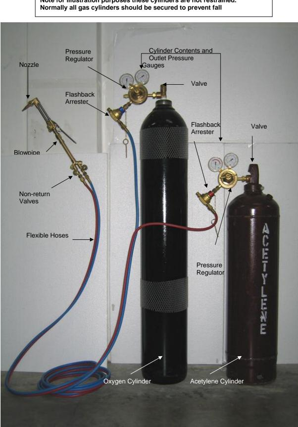
Note for illustration purposes these cylinders are not restrained. Normally all gas cylinders should be secured to prevent fall
