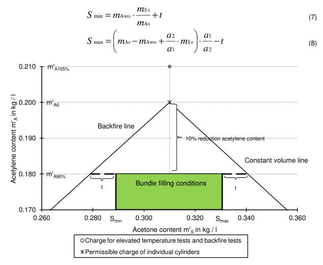
Figure 4: Example for filling conditions for acetylene cylinder bundles according to EN 12755:
