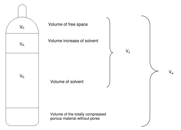
*Figure 1: Schematic description of the available volume of an acetylene cylinder* When filling acetylene cylinders, two basic considerations shall be taken into account:
