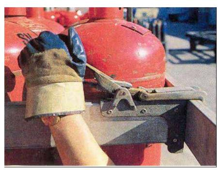
Figure 7 - Transverse slats with rapid clamping device
