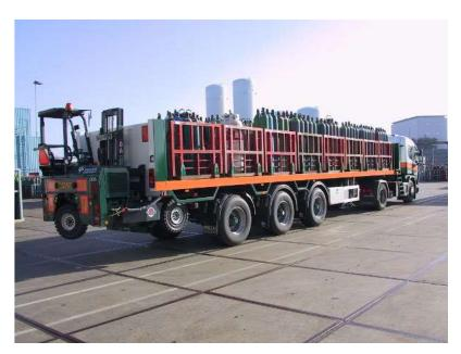
Figure 13 - Cylinder truck with forklift
