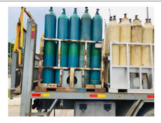
Figure 6 - Vehicle with cylinder pens and load secured by straps
