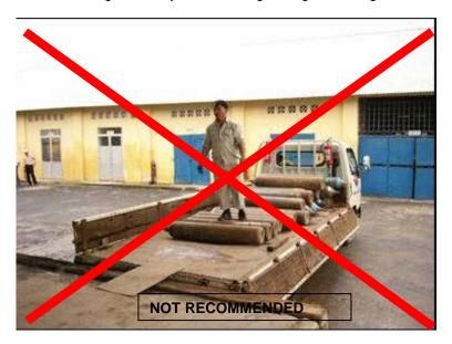
Figure 5 - Rolling cylinders by foot
