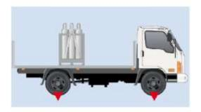
Load distribution diagrams are a valuable aid in determining the most favourable or the permissible distribution of the load. These diagrams, vary from vehicle manufacturer and model and a typical example is shown above.
