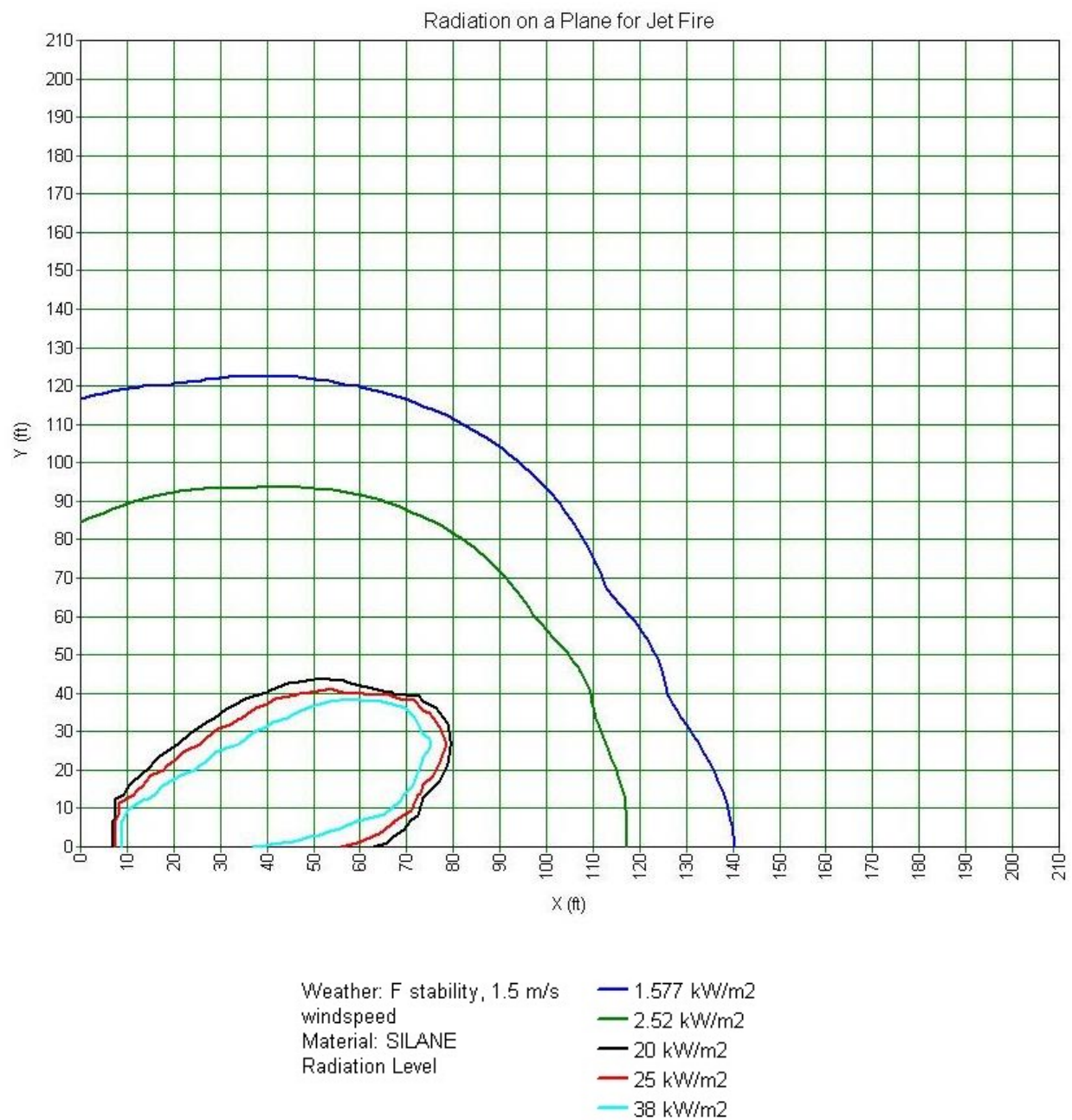
Figure D-17—Thermal radiation for ton tank (450 L) with .39 in pressure relief device, 100% flow for use
