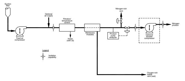
Figure 11— Typical membrane nitrogen flow diagram
