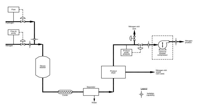
Figure 14—Typical deoxo flow diagram
