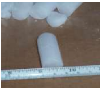
Extruded dry ice pellets (3/4 in [1.905 cm])
