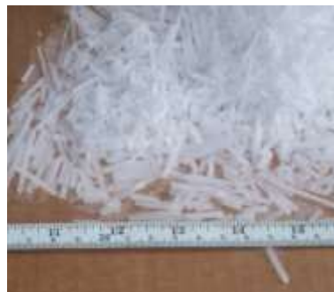
Cryo/high density/blasting ice (0.14 in [0.289 cm])
