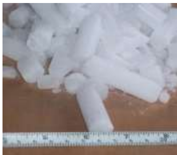
Extruded dry ice pellets (5/8 in [1.588cm])
