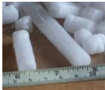
Extruded dry ice pellets (1/2 in [1.27 cm])
