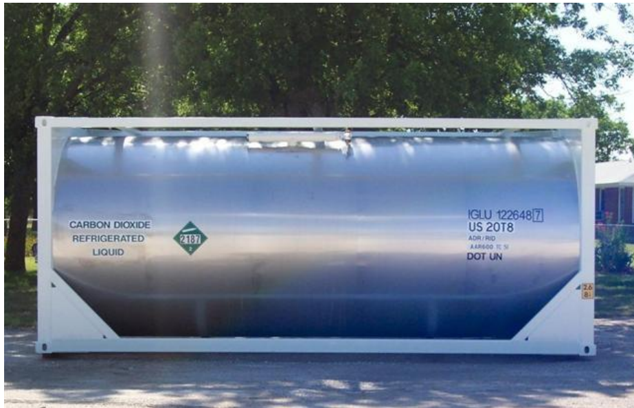
Figure A-3—Portable tank for refrigerated liquefied gas (20 ft thermally insulated container for carbon dioxide)
