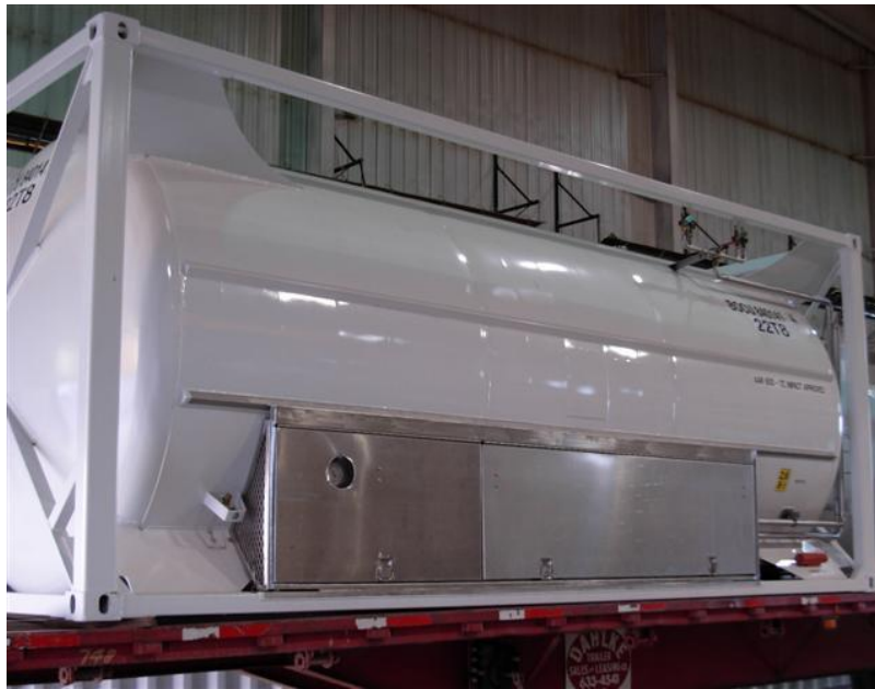
Figure A-1—Portable tank for refrigerated liquefied gas (20 ft cryogenic vacuum insulated container)
