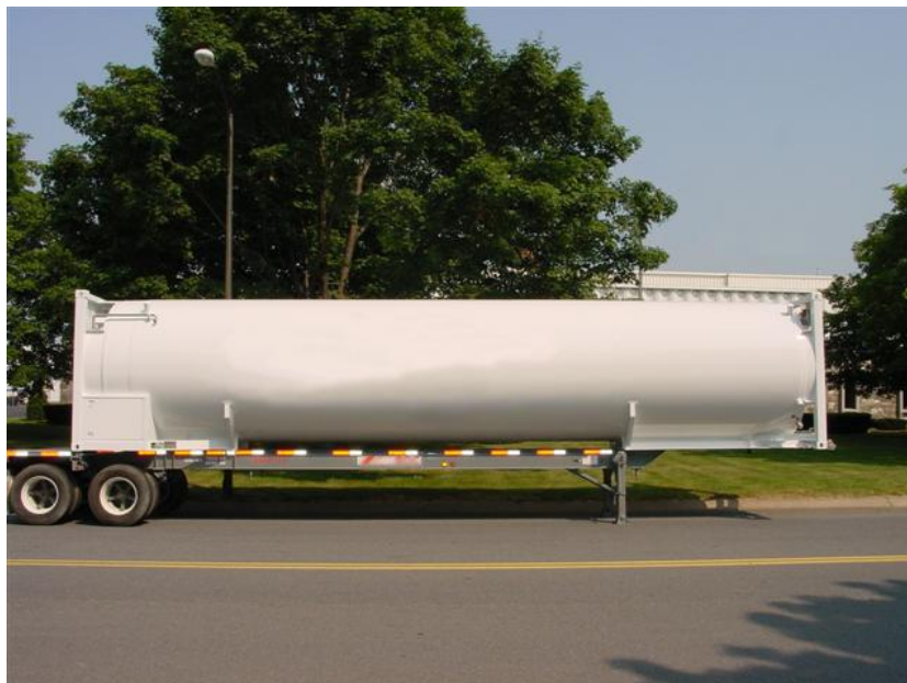
Figure A-2—Portable tank for refrigerated liquefied gas (40 ft cryogenic vacuum insulated container for helium with a nitrogen shield)
