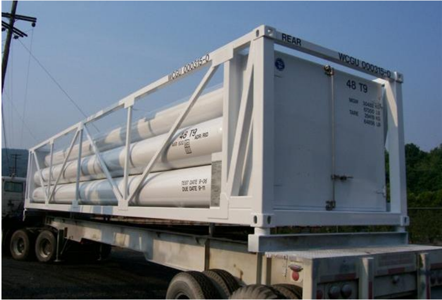
Figure A-6—MEGC (40 ft for compressed and liquefied compressed gas)
