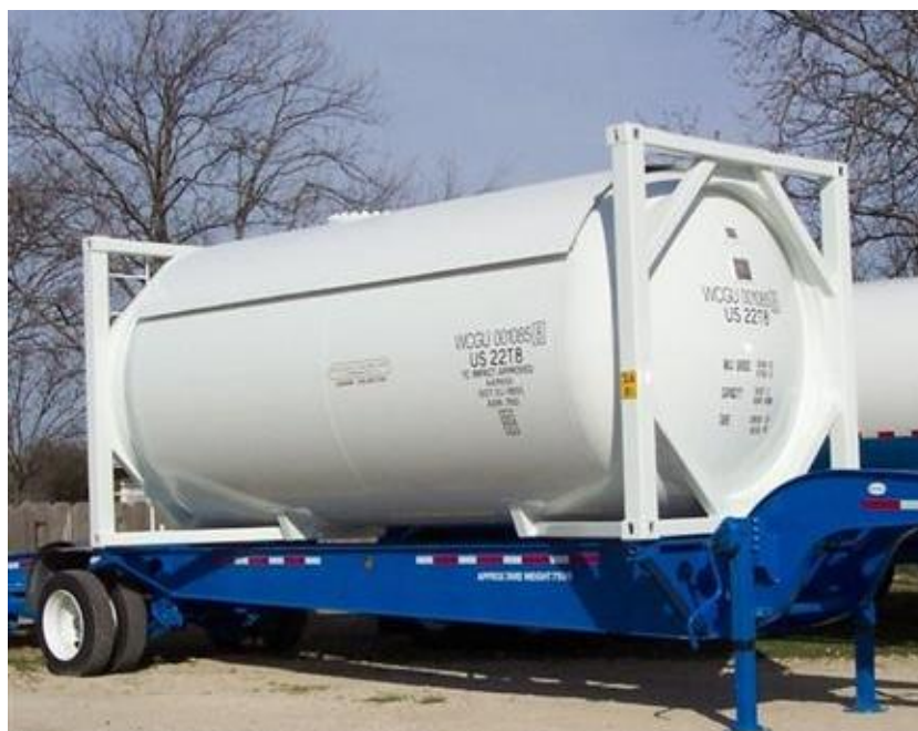
Figure A-4—Portable tank for liquefied gas (20 ft non-insulated container with sunshield)
