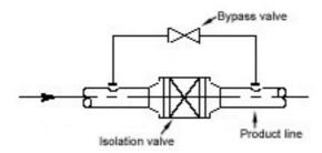
Figure 3—Example for a bypass system
