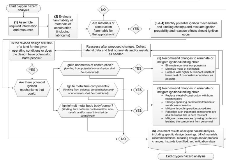
Figure 1—Flowchart showing an oxygen hazard analysis
