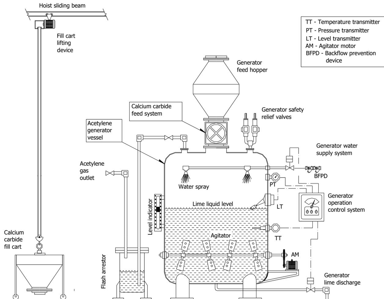
**Figure 1—Example of a wet acetylene generator system**
