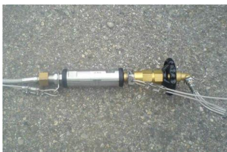
Figure 2 Typical breakaway coupling for gaseous filling
