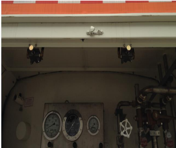
Figures B-4: Air Interlock With Round Push Button
