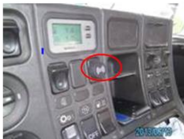
Figures B-6: In-Cab Visual and acoustic warning signs (left – visual; middle – acoustic)
