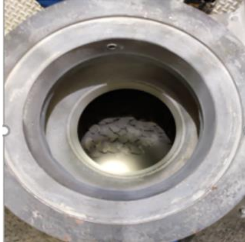
Generator hopper –no sign of internal fire
