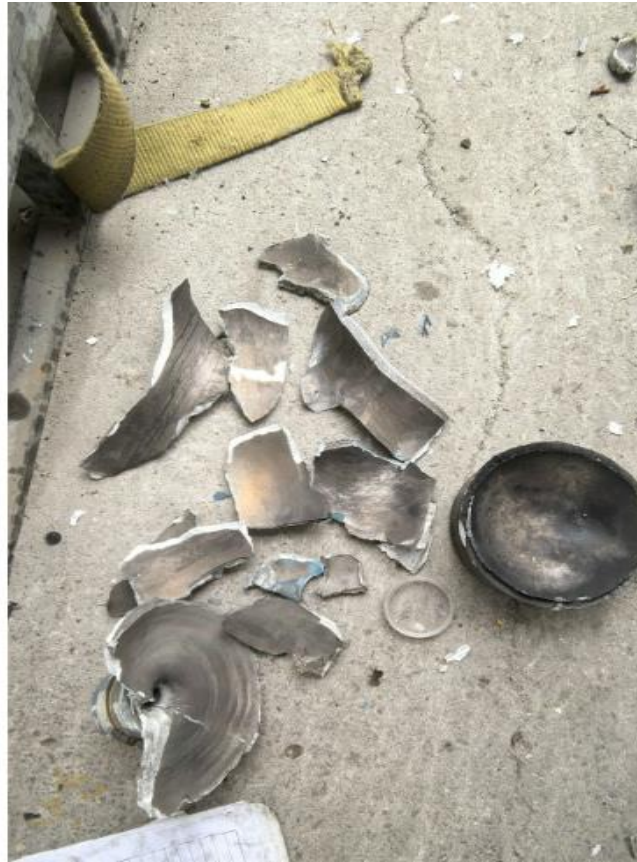
Broken pieces from ruptured cylinder
