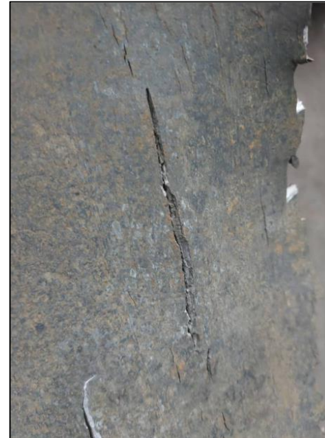
Defect on the inside of cylinder
