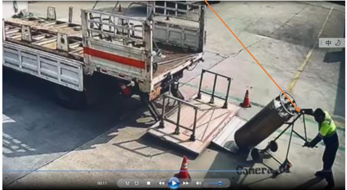
PG driver's hand placed wrongly on LGC
