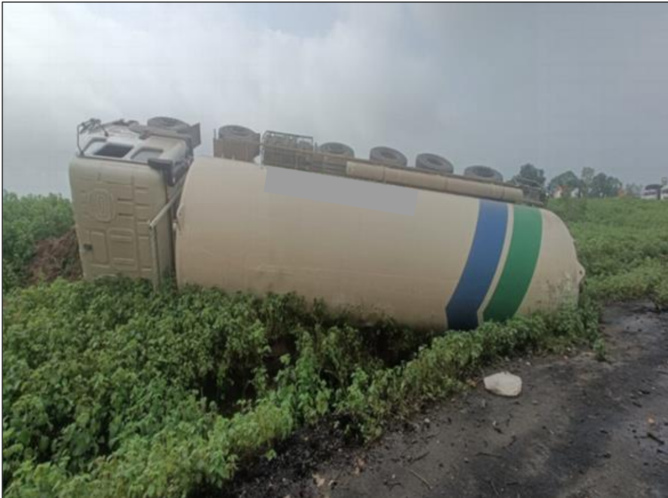
Rolled Over Tanker on soft slope ground
