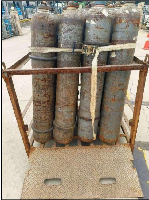
Cylinders strapped but tilted
