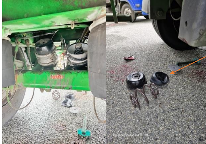
Chamber cover that hit the mechanic
