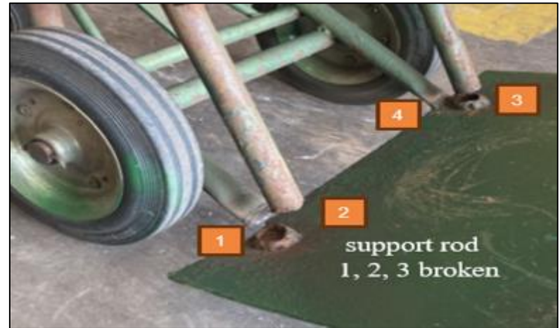
Support rods broken
