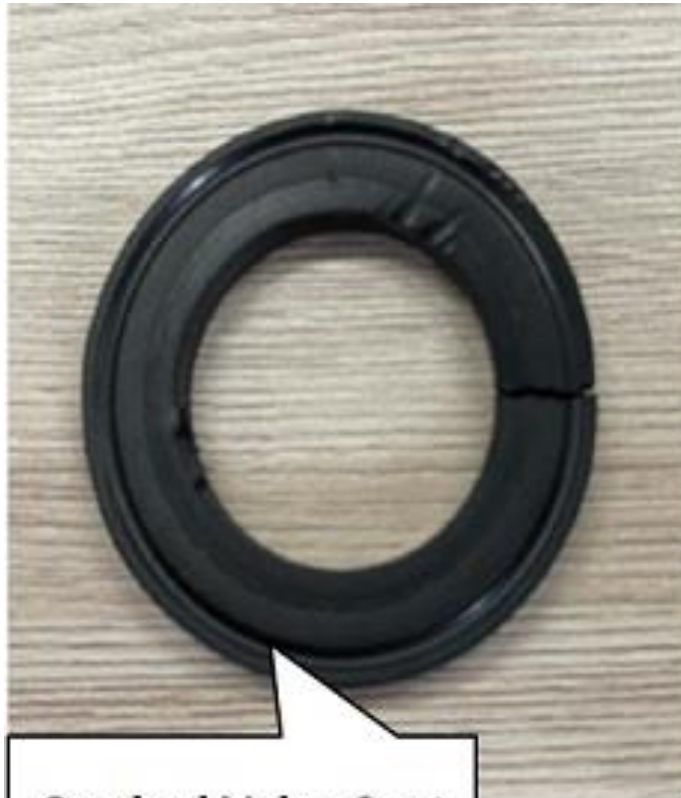
Cracked Valve Seat
