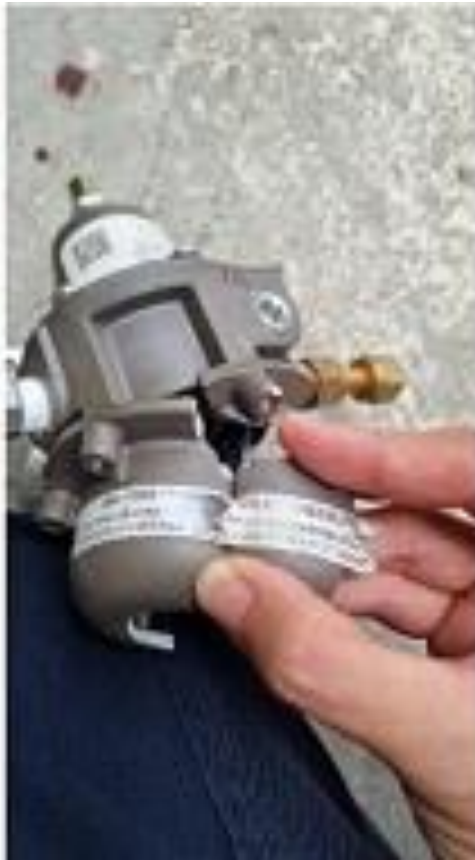
Incorrectly rated pressure regulator
