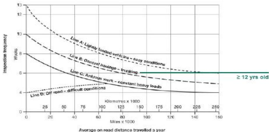
Figure 1: Example of guide to safety inspection intervals (United Kingdom Driver Vehicle Standards Agency) [3].
