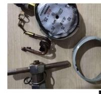
Oil can be detected under UV-light in the internal of blasted pressure gauge
