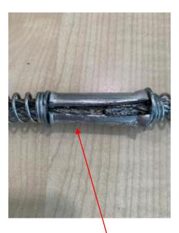
The end of the loop which was shroud on the hose neck at the tanker side gave away from the cable crimper.
