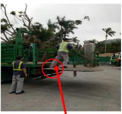
The escort's left foot slipped back to trap into the gap between tailboard and chassis, and was pinched by tailboard
