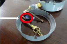
Two 4mm-diameter small hole in the back of pressure gauge, can not effectively release pressure
