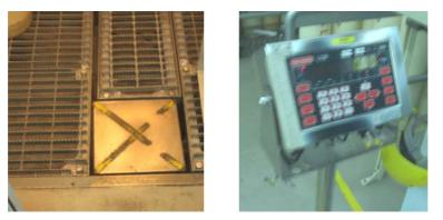
Figure 9 - Weigh scale platform and indicator
