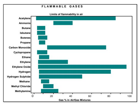
Figure 6 – Flammability ranges of gases
