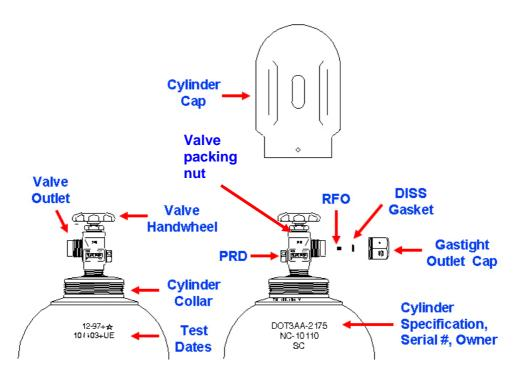
Figure 1 Cylinder parts and markings.
