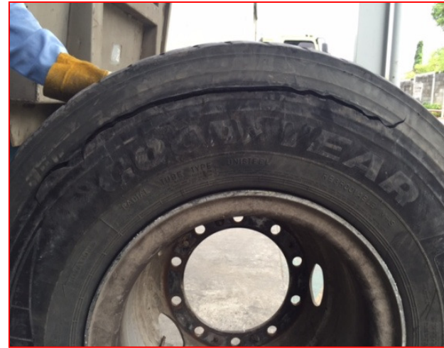
Truck's tyre burst after repair, while inflating
